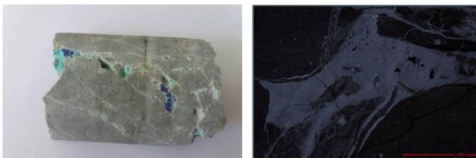
Figure 2. Polished sections: top — nests of azurite (blue) in association with chalcantite (light blue) along fractures in the core; bottom — veinlets of tenorite with mosaic twinning structure, ×50 (scale bar 500 μm)
