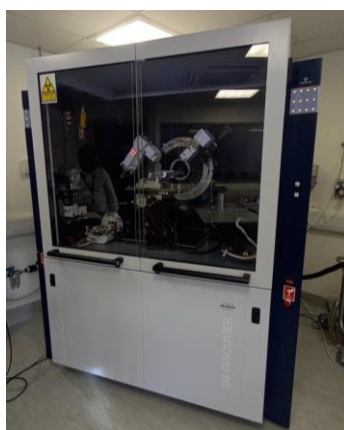
Figure 3. Photograph of the D8 VENTURE X-ray diffractometer (XRD) (Bruker) Note – compiled by the authors
