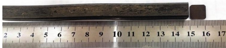
Figure 2. Appearance of titanium produced by ABC pressing and rolling, with a cross-section of 10.5 × 10.5 mm and a length of 14.5 mm
