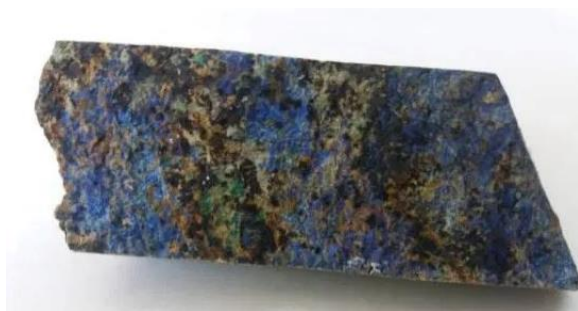
Figure 1. Polished section. Crusts of azurite (blue), malachite (green), and goethite (black) along cleavage planes of the core
