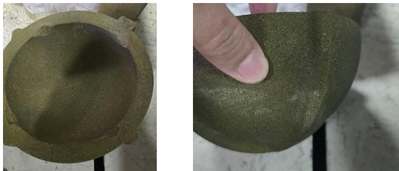
Figure 2. Molds made at the factory with the use of variable pressure
