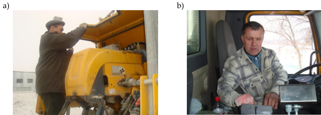
Figure 4. Regulation of chemical reagent distribution rates using (a) the external shutter of the spreader and (b) the onboard computer.
