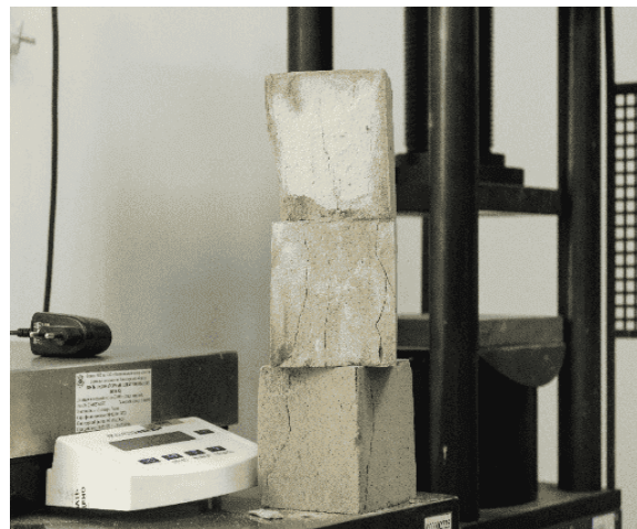
Figure 8. Compression testing of samples (cubes)– samples after the test
